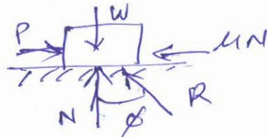
Angle of repose - The angle of inclination  $\alpha$ , at which the body slides on its own is called angle of repose.
