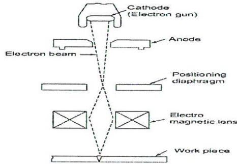
**Advantages of Electron-beam welding:**
