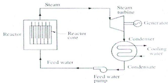
Fig. Boiling Water Reactor
