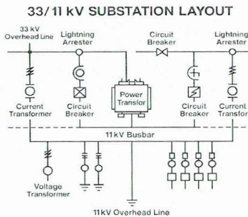
33/11 kV Substation layout showing location of all substation equipment
