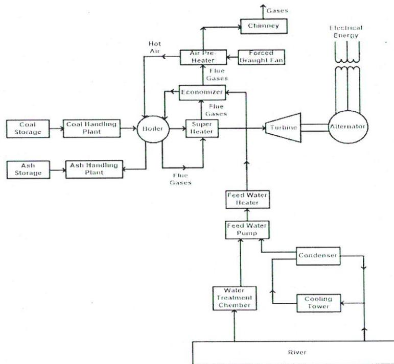
Figure: Thermal power plant Layout
