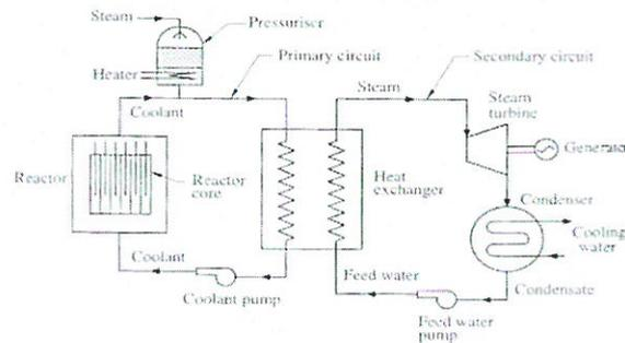
Fig. Pressurized Water Reactor.
