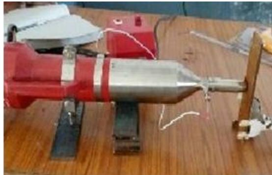
Fig 1 Pictorial view of horizontal jet on flat plate
