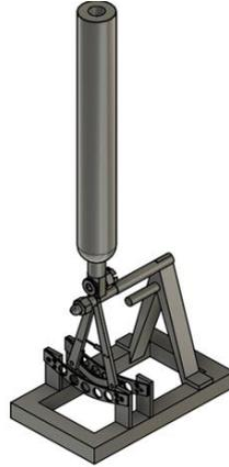
**Figure 1.** Bladeless wind turbine
