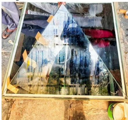
**Fig 6:** Pyramidal solar still at condensing stage.
