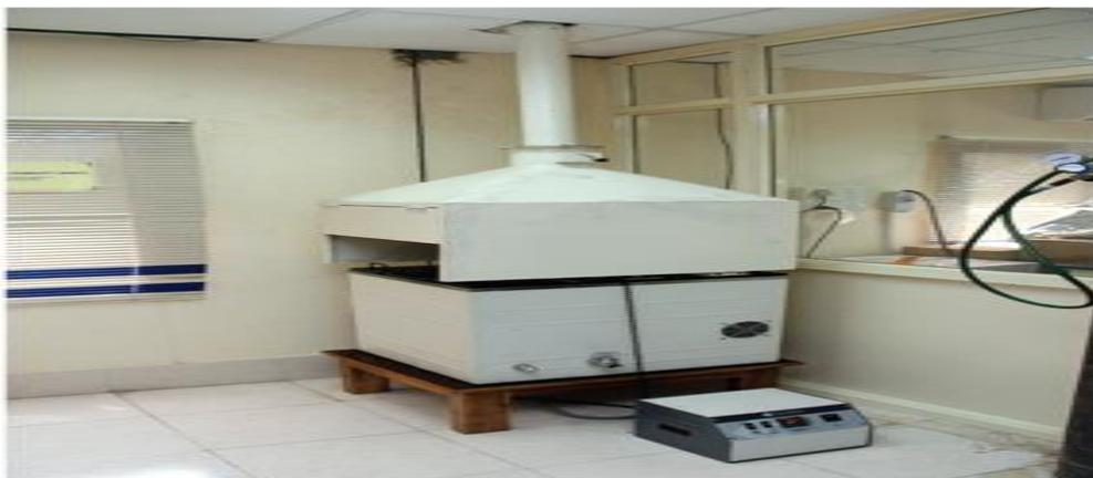
**Fig. 5.** Rotating bomb oxidation tester.
