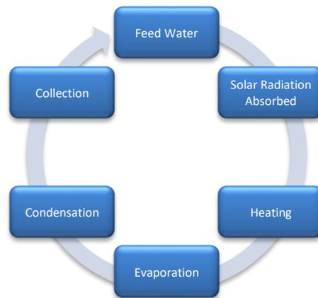
**Fig 1:** Flow chart on process of solar distillation
