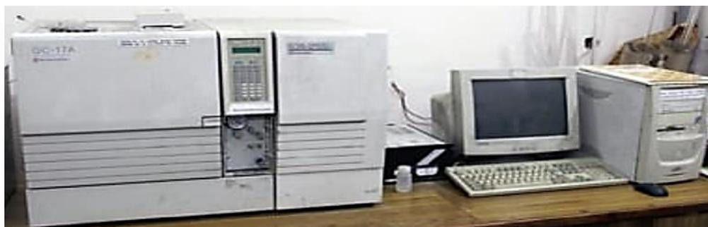
**Fig. 4.** Photographic view for gas chromatograph.
