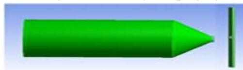
Figure 2 Horizontal jet & plate
