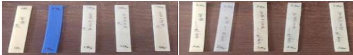
Fig 3.5 Flexural Test Specimens before testing
