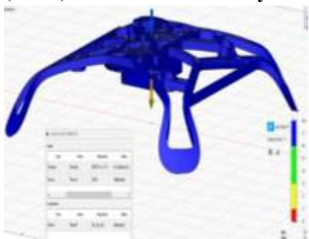
Fig-7: Center load case safety factor
