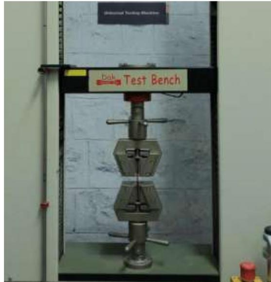
Fig. 4. Specimen Test by using Universal Testing Machine
