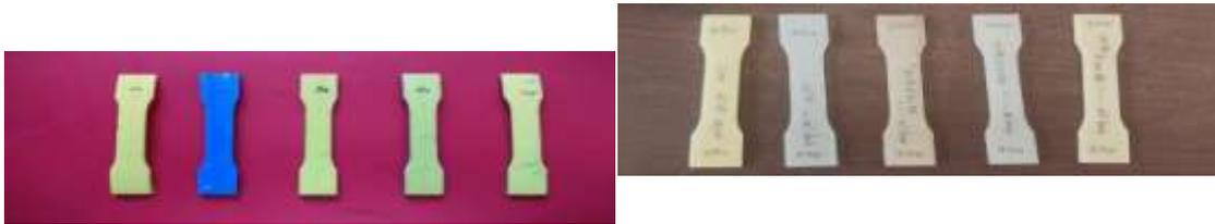
Fig No. 3.2 Tensile Specimens before Testing
