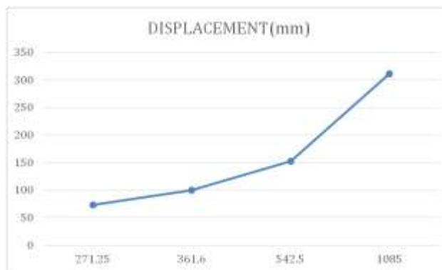
Using structural analysis, a welded plate was estimated for the Copper, at a temperature of 1085°C, displacement of the plate was obtained. By applying temperature the maximum deflection was obtained in that plate was 0.1226mm.
