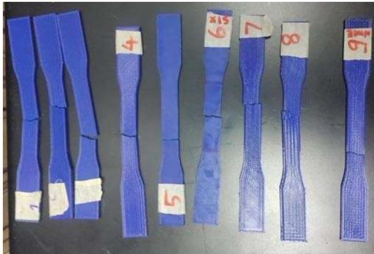
Fig. 5. Tested Specimens using Universal Testing Machine
