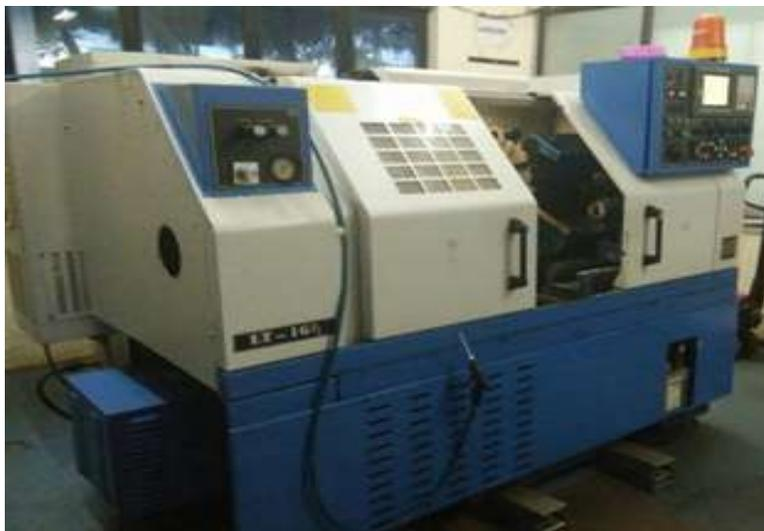
Figure 1. CNC Turret Lathe
