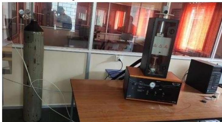
Figure 7: Thermal conductivity meter equipment and specimen
