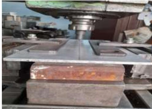
Figure 1(b) FSW tool setup
