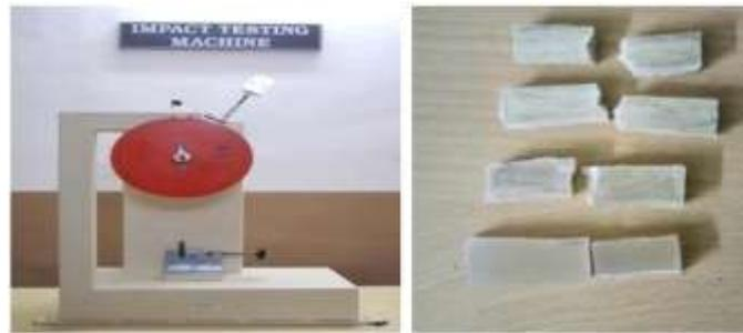
Figure 5: Impact test and fractured specimens
