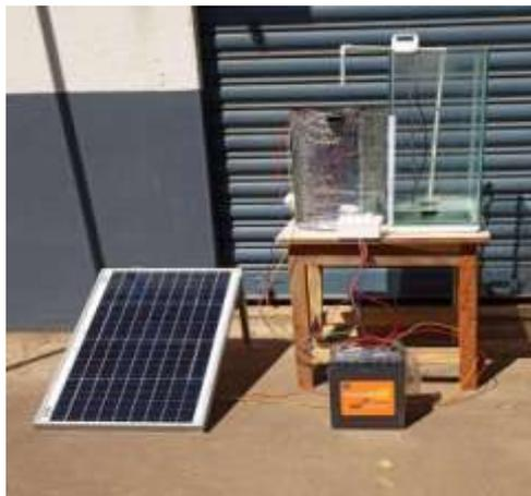
Fig 1: Fabrication of solar water heating system using solar panels and glow plugs
