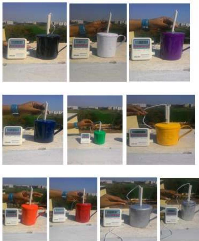
Fig1 various colours were coated to a water-filled cylinder
