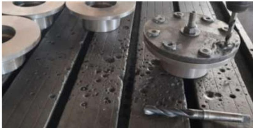
**Figure 4.** Pilot drilling of the flange using template jig
