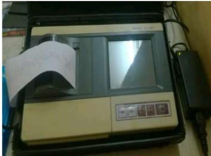
Figure 2. SJ301 Surface Roughness Tester
