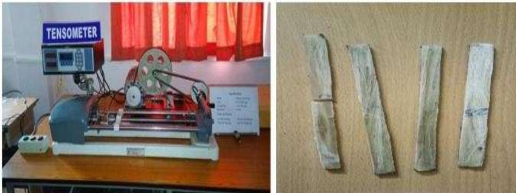
Figure 3: Tensile test and fractured specimens
