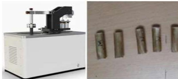
Figure 6: Pin on disc Tribometer and specimens
