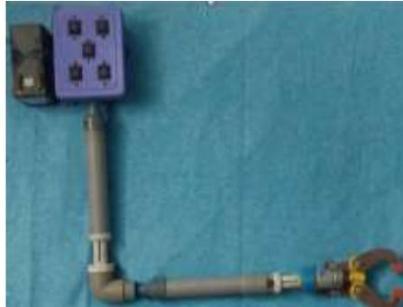
**Figure.15:** Prototype of a Multipurpose Manual Controlled Robotic Arm
