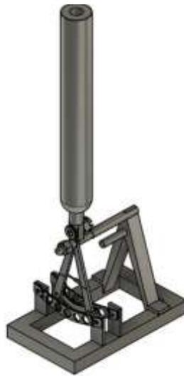
Figure 1. Bladeless wind turbine
