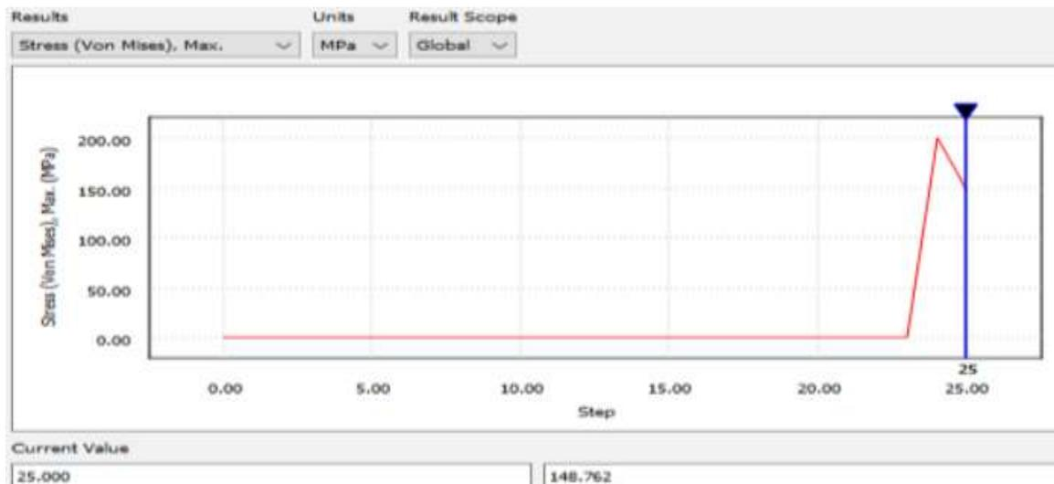
Fig-16: Graph of stress in Nylon 12(Form Labs) material
