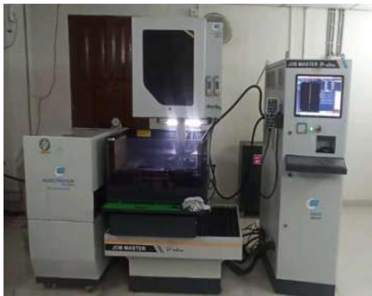
**Figure 1. WEDM Experimental Setup**
