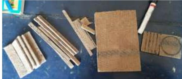
Fig 4: Cutting of composite into samples according to ASTM standards
