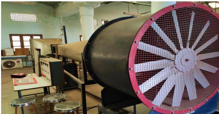
Figure 2.1 Low Speed Subsonic Wind tunnel Setup
