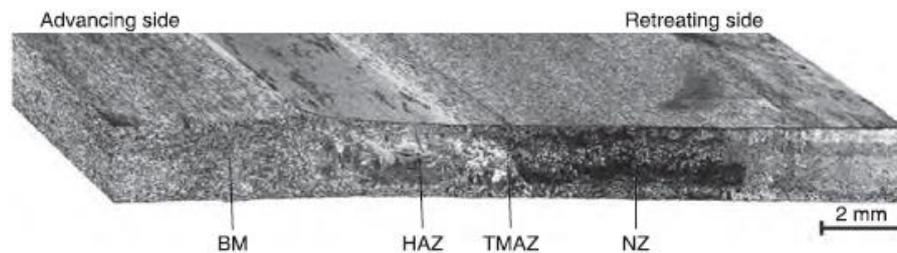
Figure-2. The microstructural zones in a friction stir welded/processed joint [8]
