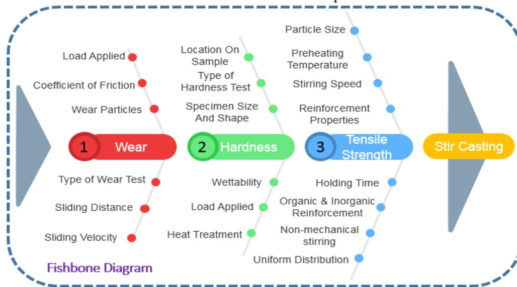
Figure 3: Fishbone diagram of factors affecting mechanical and wear properties
