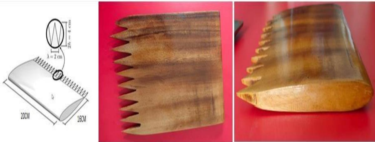
**Fig: 2.4** Schematic of a serrated wing
