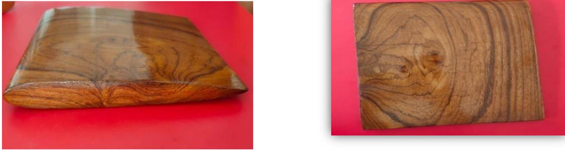
Figure 2.2 Finite wing designed and fabricated using NACA 0012 airfoil coordinates
