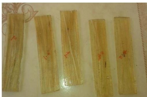
**Figure 6.** Specimens prepared for testing flexural strength
