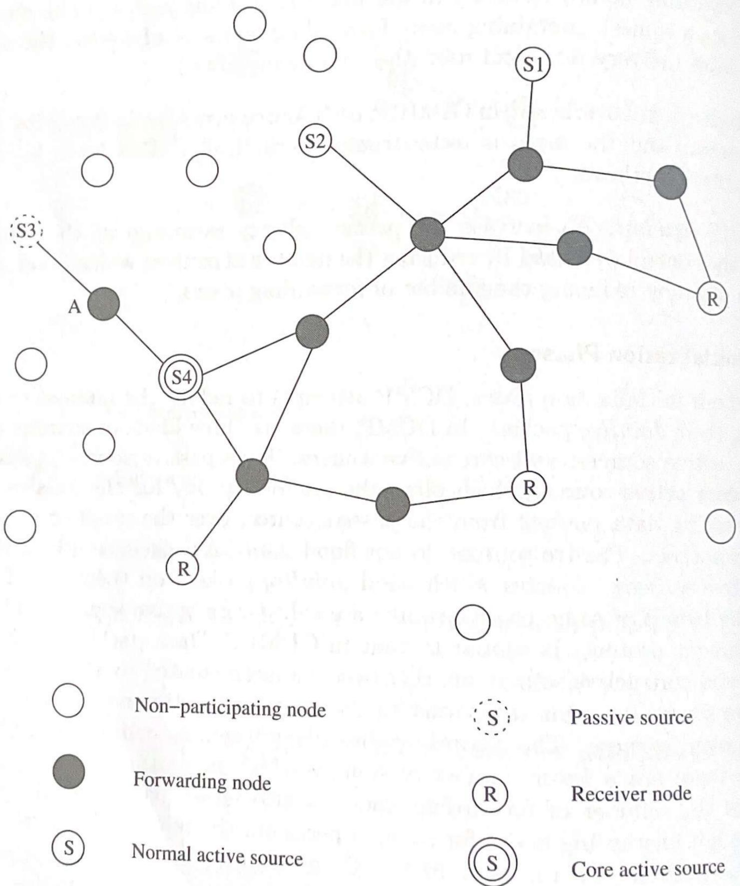
**Figure 8.32.** Construction of mesh in DCMP. Reproduced with permission from [25], © ACM, 2002.
