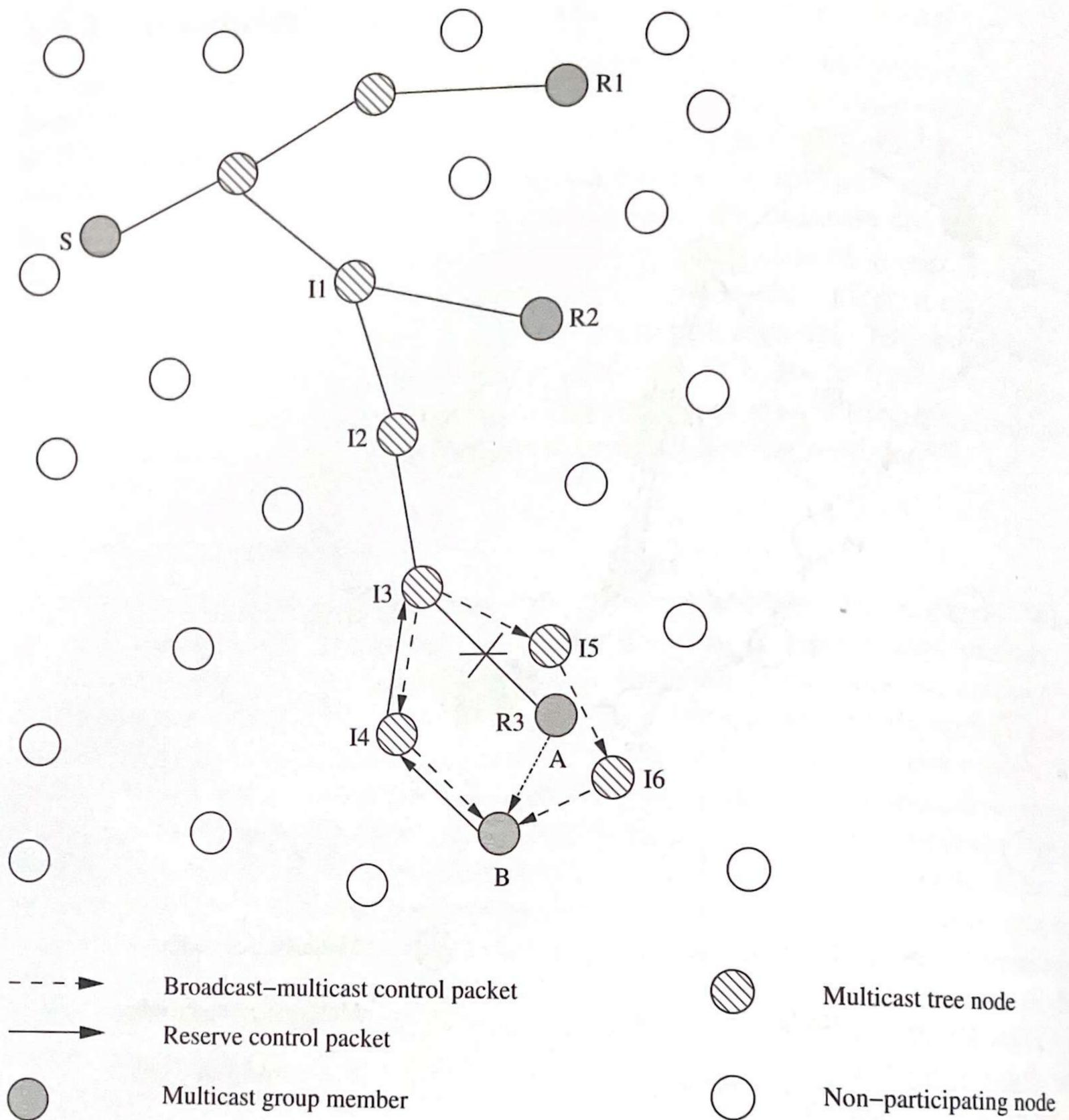
Figure 8.6. Multicast tree maintenance in broadcast-multicast scheme.
