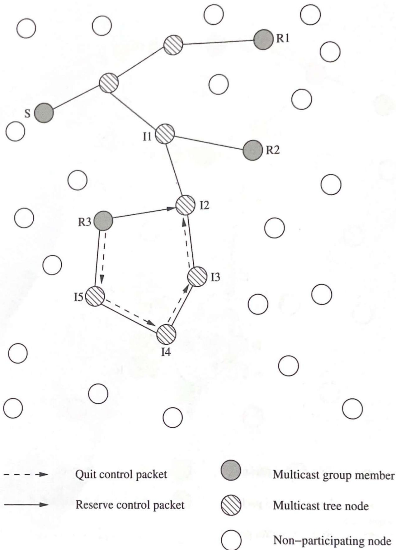
Figure 8.8. Multicast tree optimization in BEMRP.
