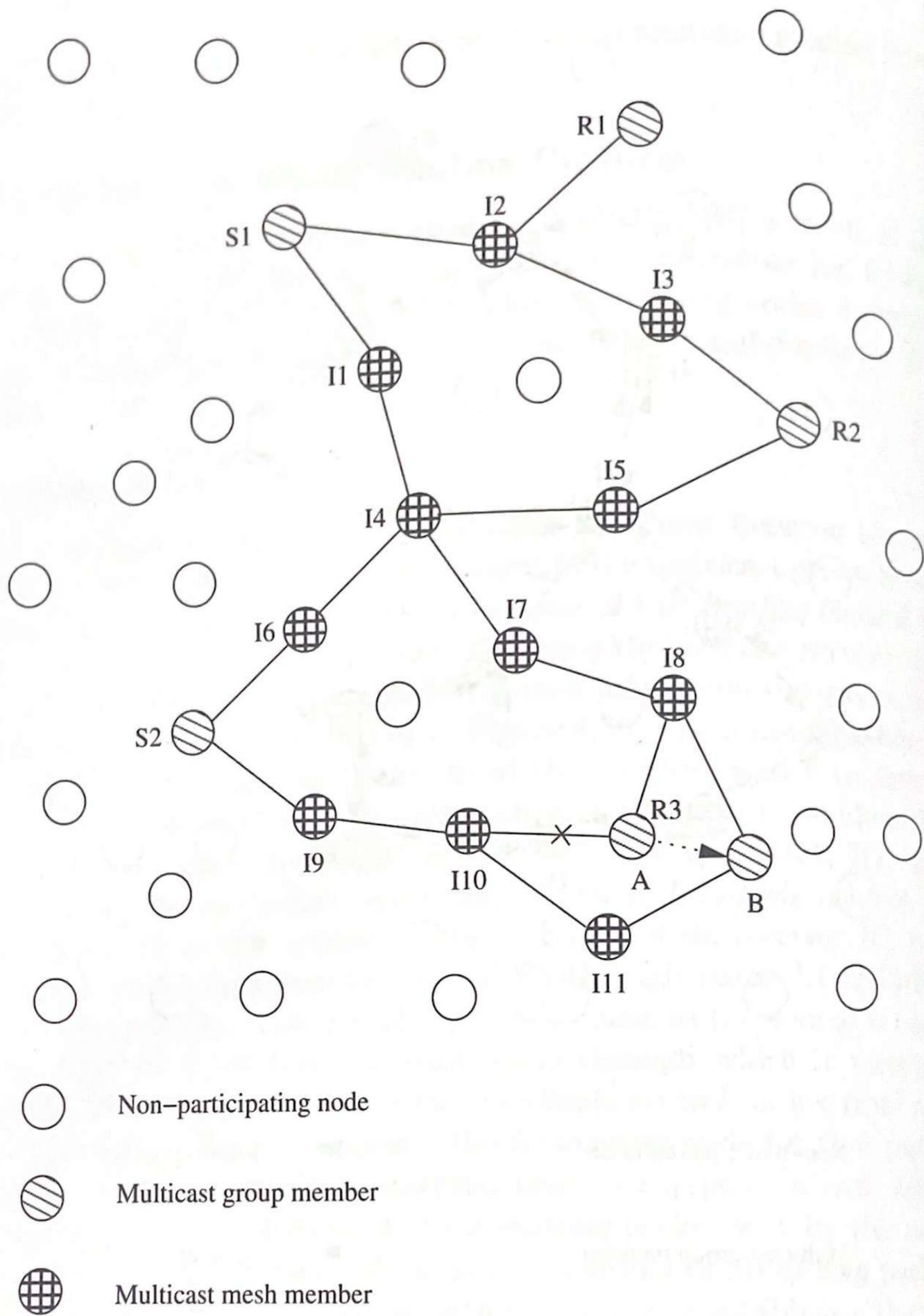
Figure 8.31. Maintenance of mesh topology in ODMRP.
