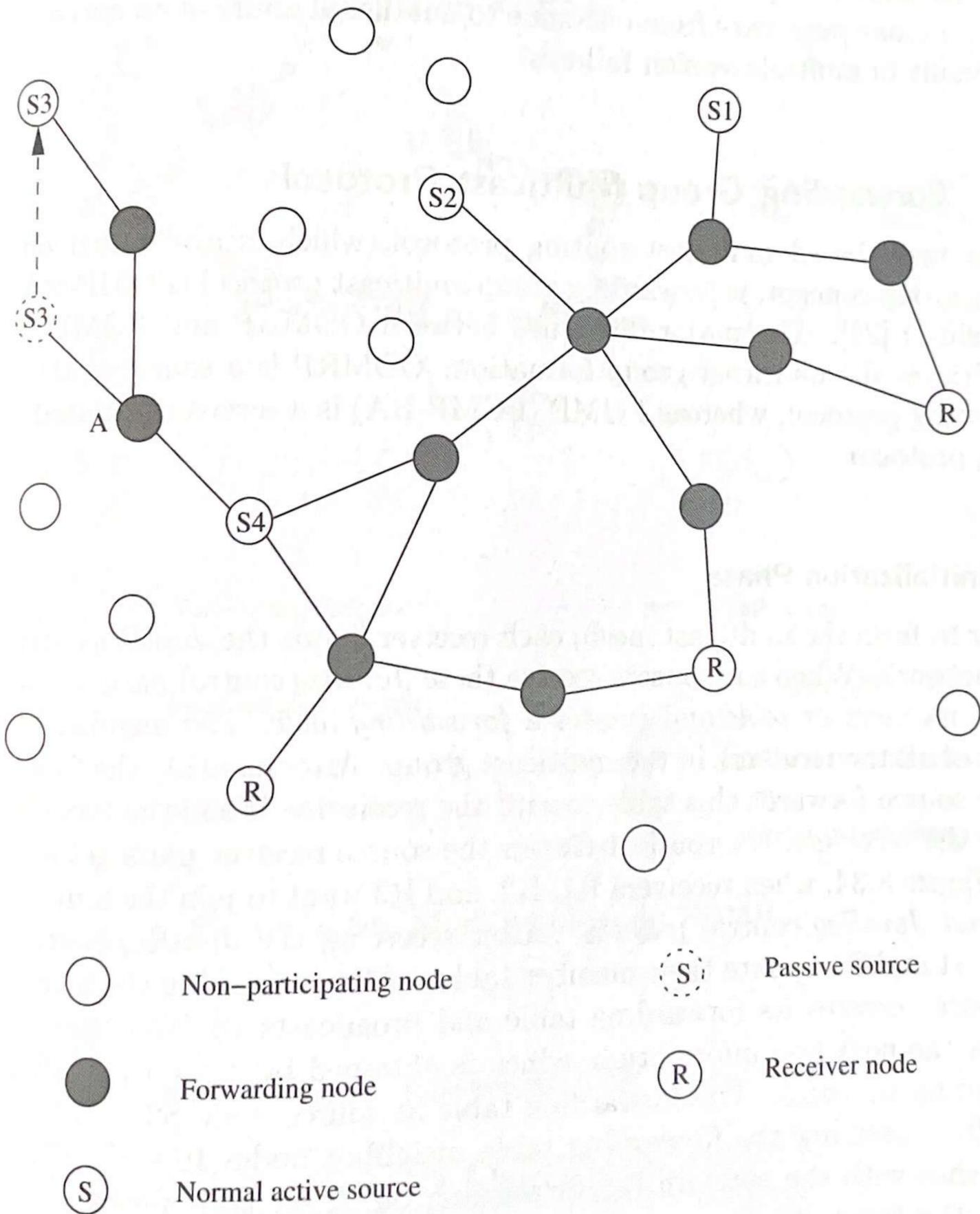
Figure 8.33. Maintenance of mesh topology in DCMP. Reproduced with permission from [25], © ACM, 2002.
