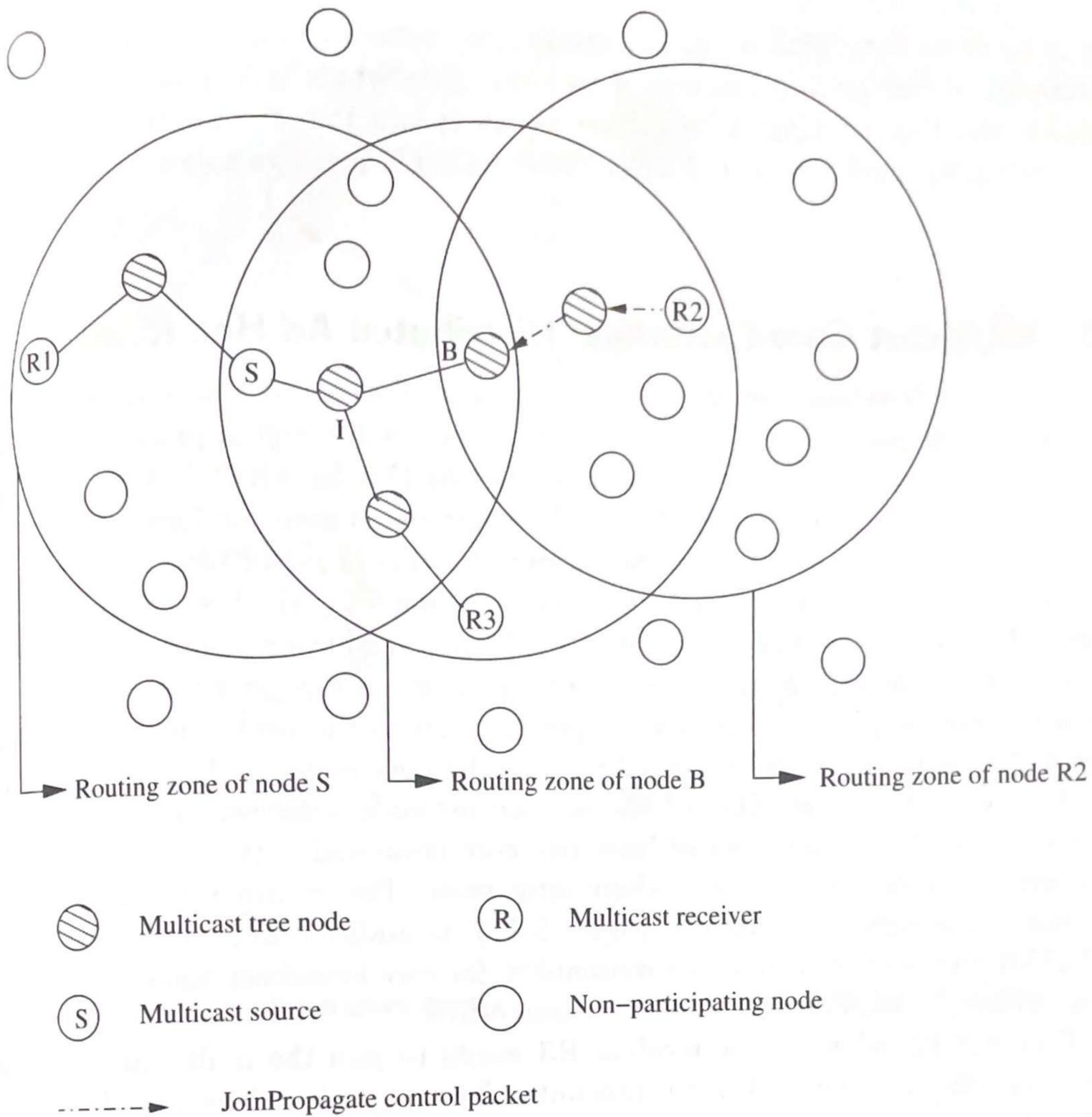
**Figure 8.11.** Multicast tree maintenance in MZRP.
