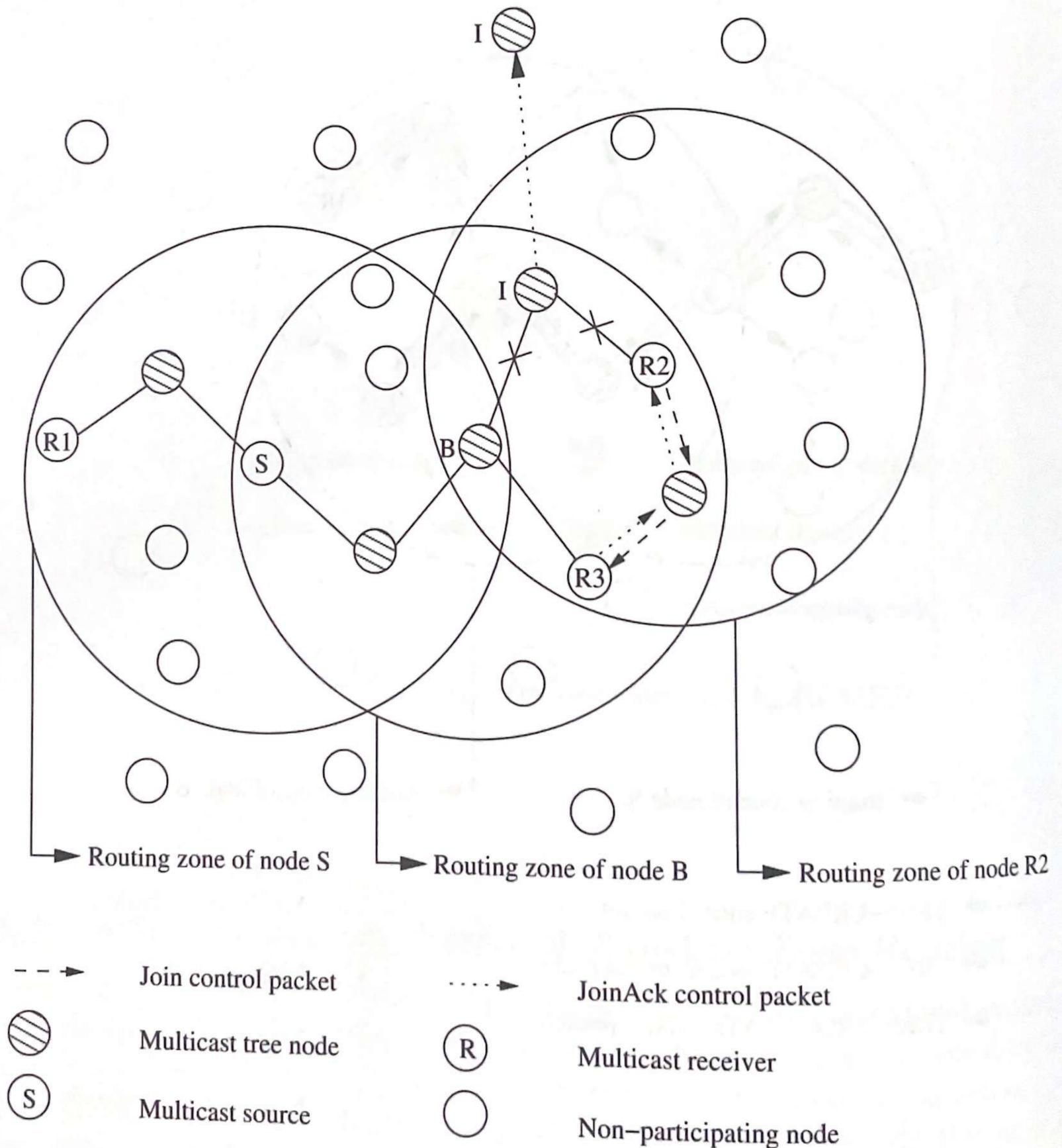
**Figure 8.10.** Multicast tree maintenance in MZRP.
