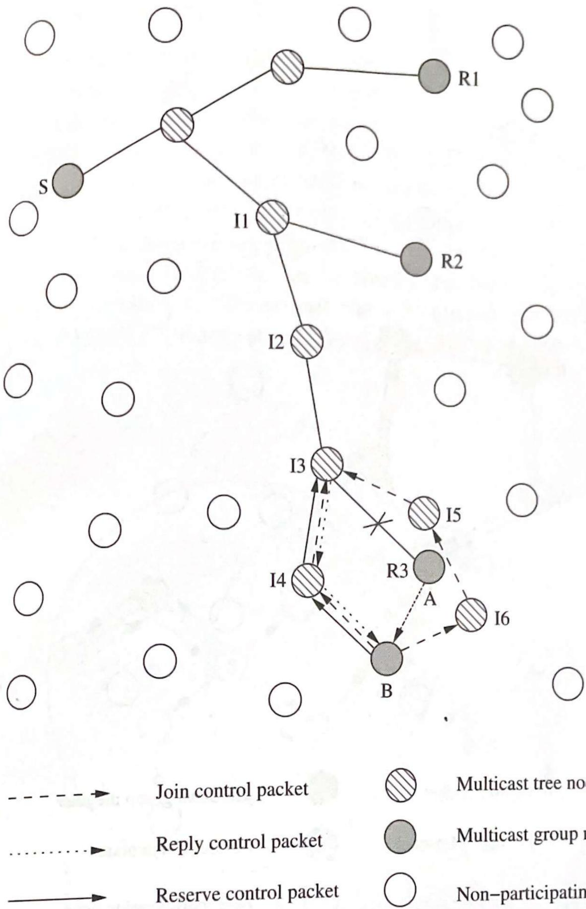
Figure 8.7. Multicast tree maintenance in local rejoin scheme.
