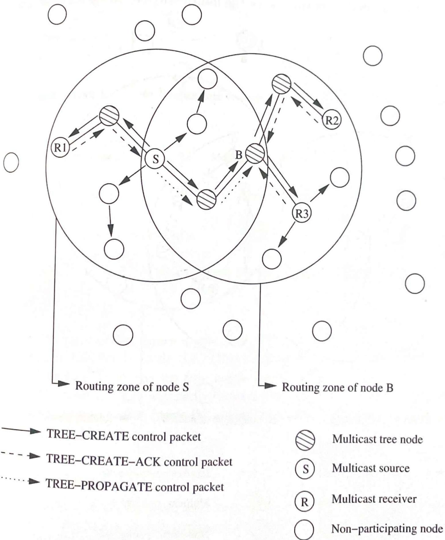
Figure 8.9. Multicast tree initialization in MZRP.
