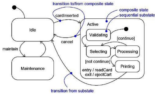
Figure : Sequential Substates
