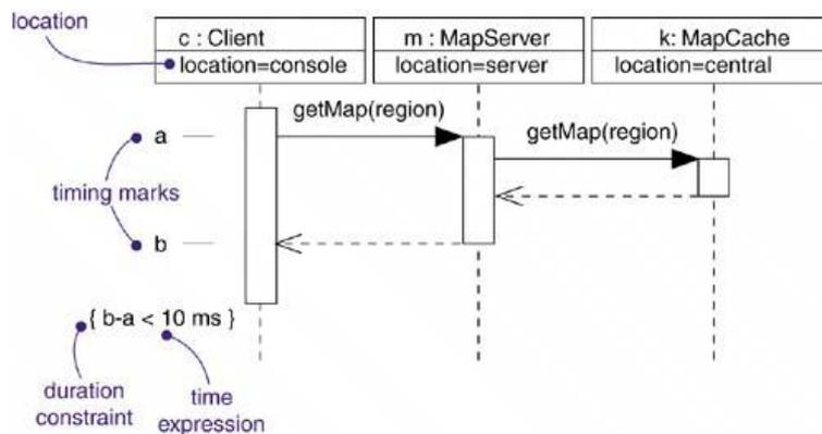
A timing mark is a denotation for the time at which an event occurs. Graphically, a timing mark is depicted as a small hash mark (horizontal line) on the border of a sequence diagram.
