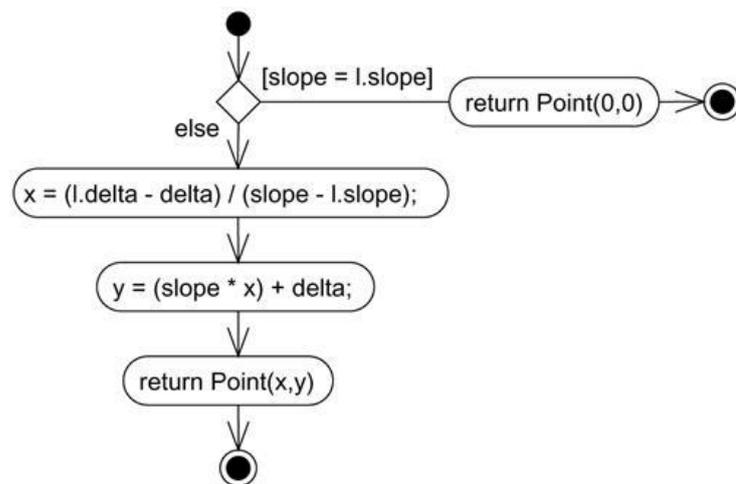
Figure 10: Modeling an Operation
