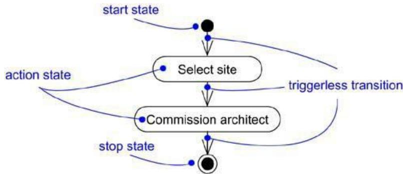
Figure 4: Triggerless Transitions
