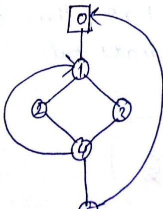
Backward edges are  $5 \rightarrow 0$  and  $4 \rightarrow 1$  and reduce or eliminate backward edges from the flow graph. Now the flow graph can be represented as
