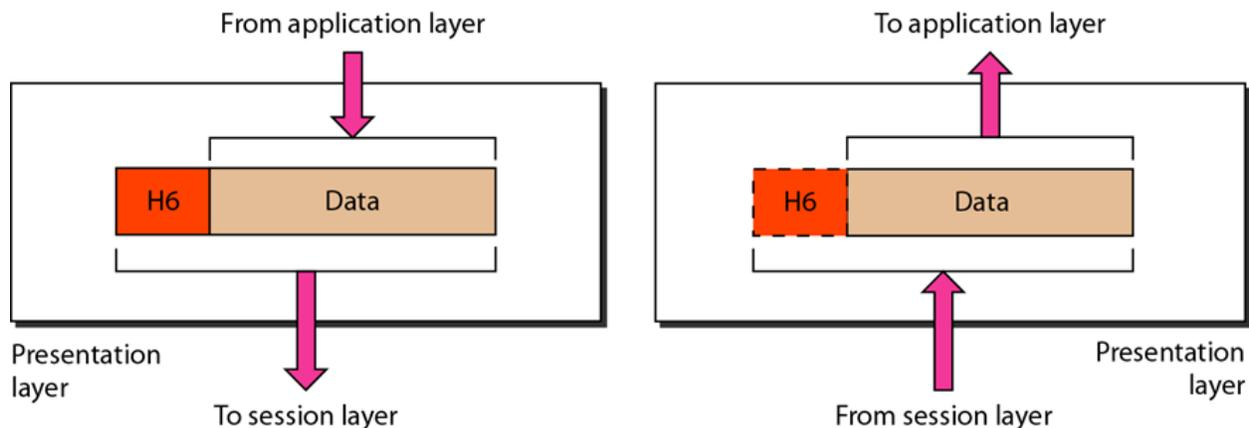
➤ **Translation-** The sending and receiving devices may run on different platforms (hardware, software and operating system). Hence it is important that they understand the messages that are used for communicating. Hence a translation service may be required which is provided by the Presentation layers
