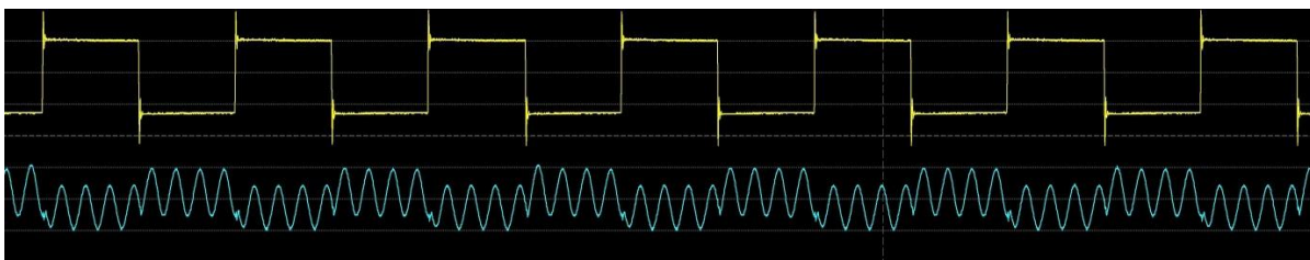
Figure 2: I/P data & Modulated O/P
