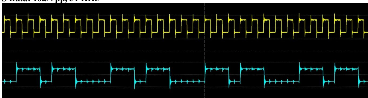
Figure 2: Clock & Serial Data
