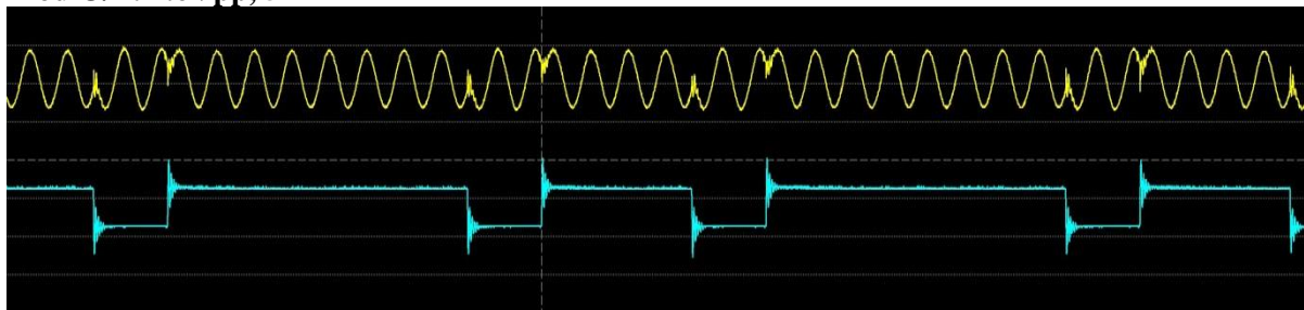
Figure 3: Modulated O/P & Differential Data
